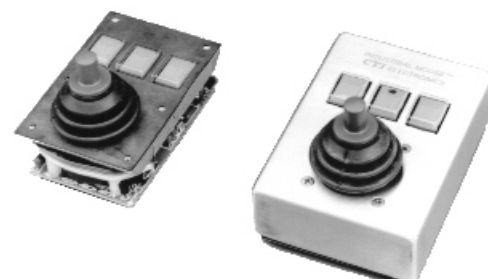
The CTI Electronics Industrial Mouse™ Panel Mount (H2 Series) on left Hand Held (M2 Series) on right
